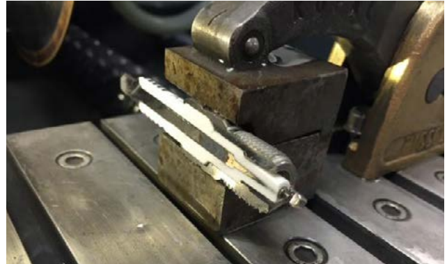
Exhibit 1: The final result from cutting a spark plug in half with minimal mechanical damage to the specimen.
