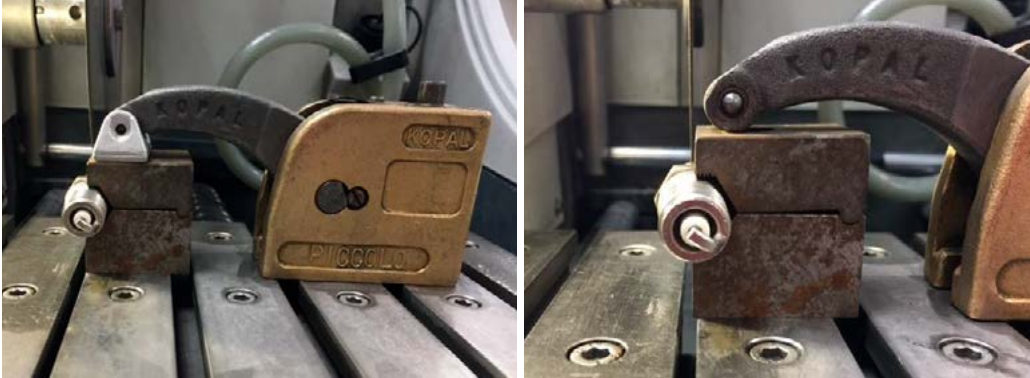
Exhibit 2: Using a special clamping tool and dedicated vise. The use of swivel shoe on the clamp showed no significant differences in the quality of the cut.
