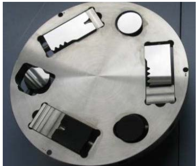
Exhibit 5: A customised specimen holder for grinding and polishing 6 differently-shaped specimens is applied.
