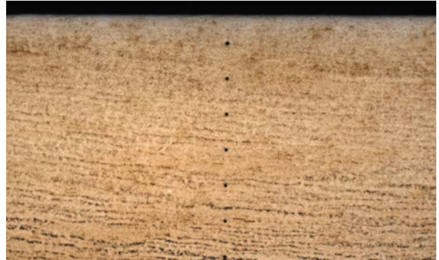
Exhibit 1: A final result of hardness testing using an automated Case Hardness Depth (CHD) process
