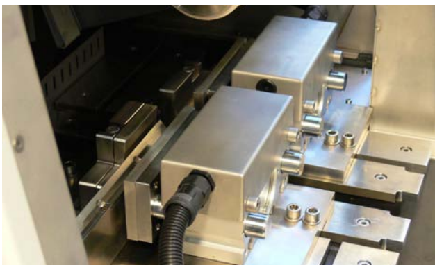
Exhibit 4: The cutting equipment is modified with an auto-feed system that eliminate manual clamping procedures and results in a tact time of 1 minute per cross sectioning
