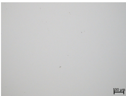
Surface after polishing with MD-Plus & DiaPro Plus 3 µm (x 100)
