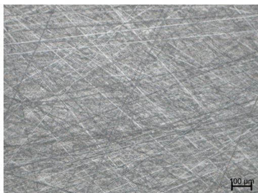
Surface after Plane grinding with MD-Diamond Pad 800 (x 100)
