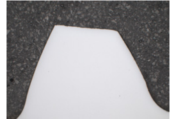
1 minute of oxide polishing with MD-Chem and OP-U NonDry 0.04 µm (x50)
