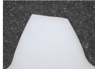
3 minutes of polishing with MD-Dac and DiaPro Dac 3µm (x50)
