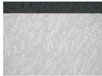
3 minutes of polishing with MD-Dac and DiaPro Dac 3 \mu\text{m} (x200)
