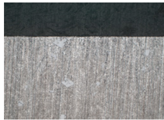
3 minutes of fine grinding with MD-Largo and DiaPro Allegro/Largo 9 \mu\text{m} (x200)
