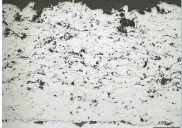
2 Plasma-sprayed molybdenum coating
