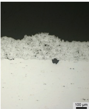
1 No delamination after cutting
