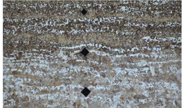
Exhibit 1: A surface prepared for hardness testing with an automated series of indentations.
