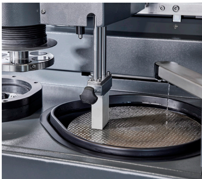
Dressing MD-Piano with an aluminum oxide stick.
