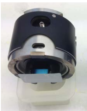
Exhibit 3: Mounting the sample into sample chair.
