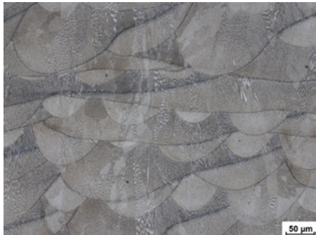
Fig. 25: Inconel 718, etched with Adler etchant. Bright field.
