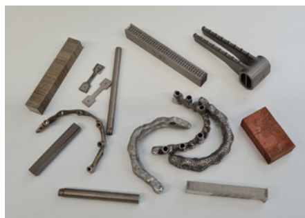
Fig. 8: Variety of metallic samples made by additive manufacturing (laser melting processes).
