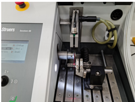
Fig. 12: Clamping of AM titanium sample in Secotom-60
