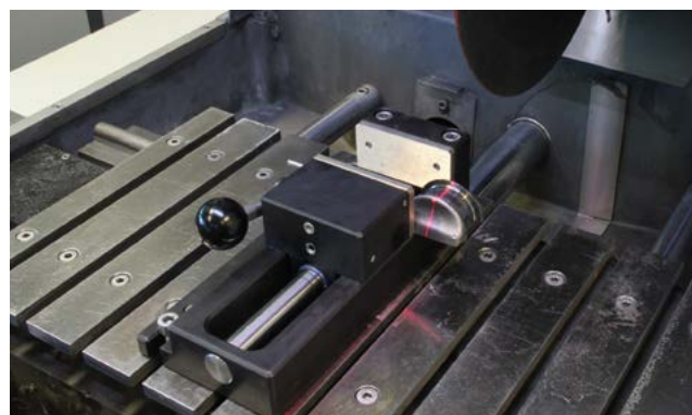
Exhibit 9: Final cuts are made with a baseplate clamp.
