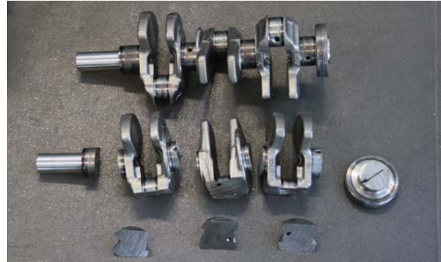
Exhibit 1: The result of 13 cuts to produce the required specimens for hardness testing.
