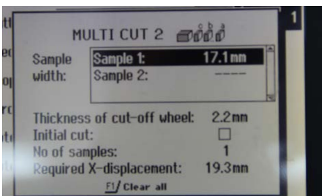
Exhibit 8: Cutting program for cutting the bearing surfaces.
