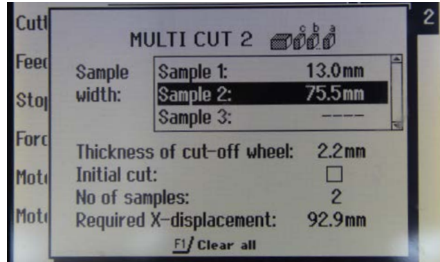
Exhibit 5: Cutting program for cross sectional cuts.
