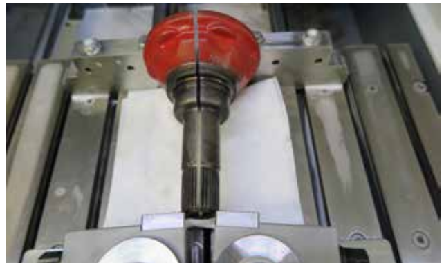
2. Clamping with a non-pinch clamping device
