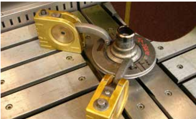
1. Large part clamped in an Axitom-5
