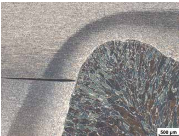
7. Preparation of weld for microanalysis, polished, etched with nital
