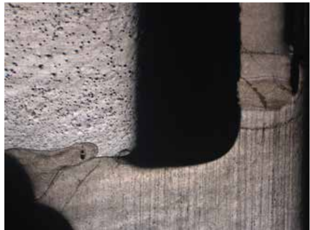
10. Laser weld, electrolytically polished (A2) and etched with oxalic acid (10%)
