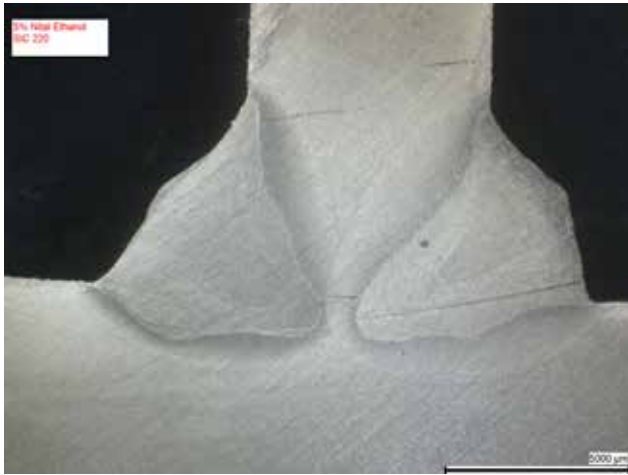
5. Macro-weld etched with nital, ground one step
