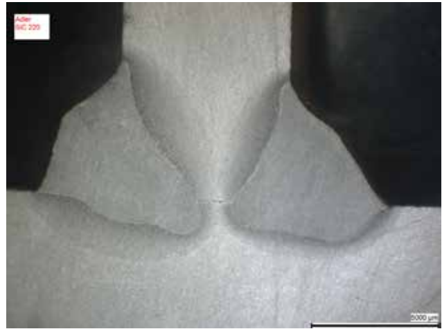
6. Macro-weld etched with Adler etchant
