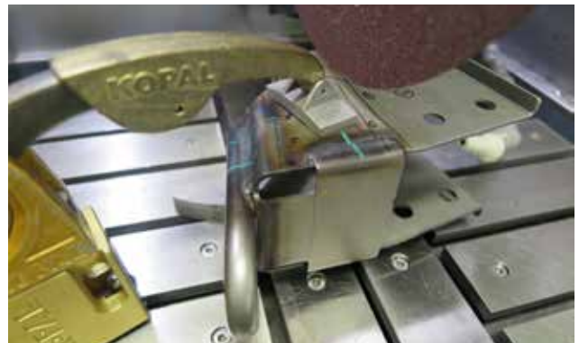
4. Clamping larger welds
