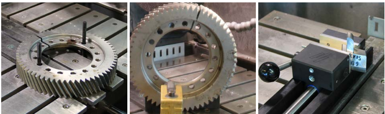
Exhibit 2: How to use special clamping setups to avoid pinching the cut-of wheel and to meet the need for the right cuts both parallel and perpendicular to the teeth surface.
